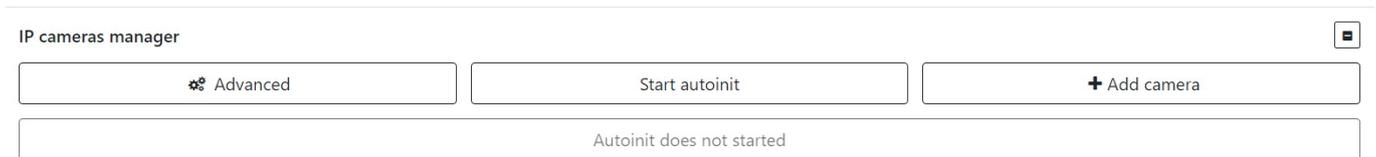
In most cases, autoinit will detect and add the camera for you, however, if this does not happen, you can try to add it manually by clicking the **“Add”** or **“Advanced”** button and specifying the desired parameters.
