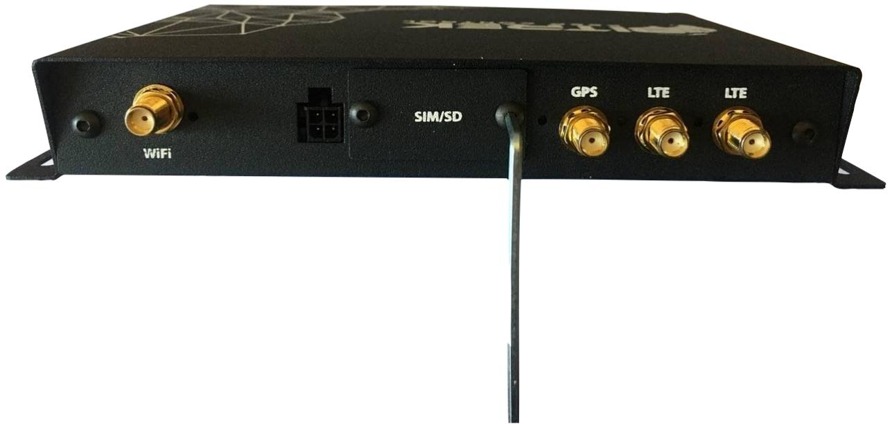
2. After installing the SIM card, connect the antennas to the device:
