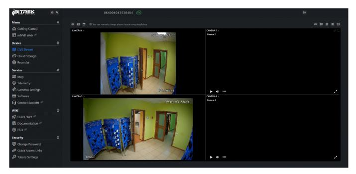
• Single-user multiple streaming video player - allows you to view images from **one** camera in live mode, other cameras will be paused to save traffic (the camera 3 on is paused in the photo)
